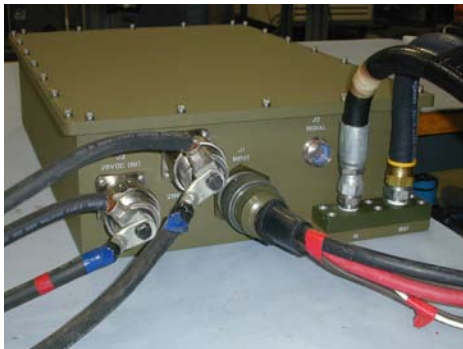
Figure 5. DRS-TEM 10kW High Voltage to 28VDC Converter
